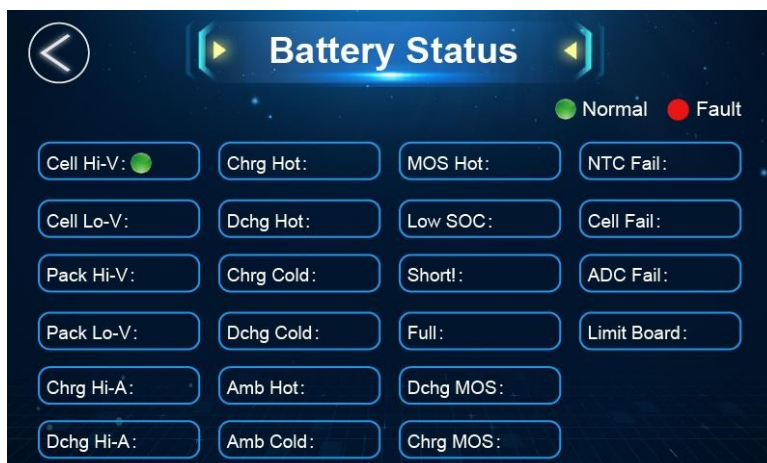
Figure 11: E300 screen; Status page for battery operational status.
