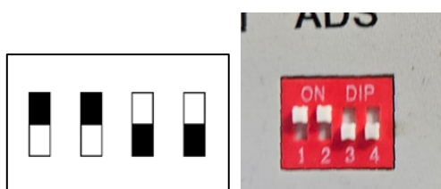
Figure 8: Dip switches on the BMS. In the image the bits are set for a slave BMS 2.
