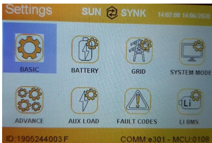
Figure 1 Settings Screen in the LCD display of the inverter showing Firmware code e301-MCU:0108 for a 5kW Sunsynk.
